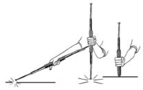
To close, simply tap the end at an angle and strike down firmly on a hard surface. Repeat steps on other side.
